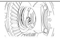
12. Push in axle and insert second Cclip thru slot in driver/spacer.
