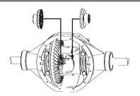
6. Install couplers, ring gear side first. Install C-clip on ring gear side only.
