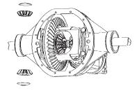
4. Rotate wheel to remove spider gears.
