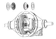
5. Remove side gears, and for limited-slip differentials, remove friction plates.
