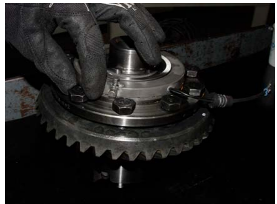
Eaton ELocker™ differential (Selectable between open and locked modes)
